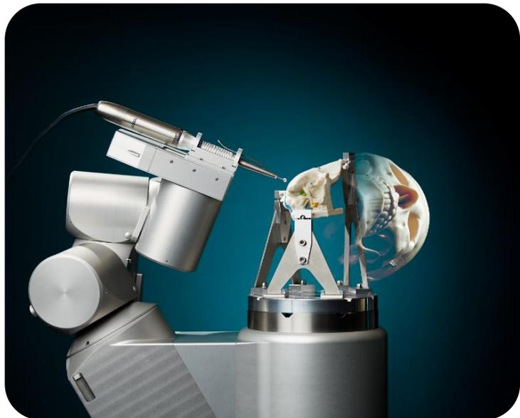
The robot will be able to autonomously carry out instructed tasks, but can also be operated manually using a haptic device. This haptic device allows the surgeon to be in full control of the movement of the robot while getting force feedback. Tremors and other unintended inputs are filtered.
